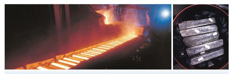
Electralloy supplies AOD refined, 15 lb. pigs with certified analysis. Electralloy can also reclaim scrap, gates, risers and miss-runs, melt, AOD refine and cast 15 lb. pigs with certified analysis to specified chemistry.
