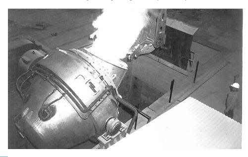
Electralloy supplies the casting industry with AOD refined, 15 lb. pigs with certified analysis. Electralloy can also reclaim scrap, gates, risers and miss-runs, melt in their arc furnace, refine in AOD units, and cast 15 lb. pigs with a single certified analysis for heats up to 52,000 lbs.
